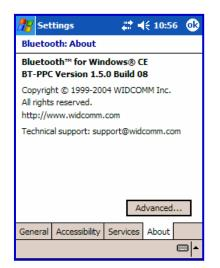
16. To determine the version of the Bluetooth stack installed on your handheld device, locate the Bluetooth icon and tap it with the stylus to open the application. Find the Bluetooth About tab and tap to open the associated page. There you will find the version and build for the installed Bluetooth stack.
